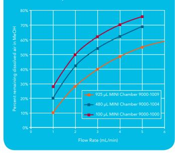
Plot shows remaining dissolved air in methanol using a selection of Systec Mini-Chambers\*. The range of chambers and specifications offered provide ample solutions for system designs.
