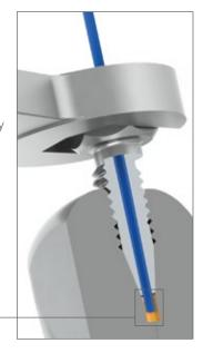
MarvelXACT fittings do not depend on ferrules. They seal at the bottom of the port, without complex techniques, which significantly reduces required torque and enables many more connects and disconnects. MarvelXACT significantly reduces wear on your hardware, increasing product life. An enhanced proprietary tip design also ensures zero dead volume (ZDV) and better chromatography results.
