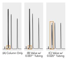
Conclusion: These sequential chromatograms show the effect of adding volume to the flow path through the addition of components.
