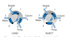
Flow path of Two-Position, Six-Port Injection Valve
