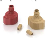
Two-Piece Fingertight Fittings feature a separate ferrule. Use a standard knurled head fitting for traditional fingertight applications, or use a fitting with wings built into the head for extra tightening leverage. A stainless steel hex headed fitting can be used for applications where a wrench may be needed for added tightening torque.
