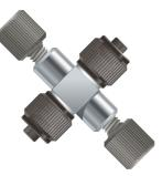
VHP MicroTight Adapting Cross 10-32 Coned for 1/16" OD tubing and 5/16-24 Coned for 360 µm OD tubing
