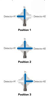
**Characteristics of Manual Sample Injection Valves**
