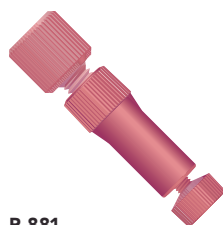
P-881 MicroTight ZDV Adapter for 1/16" to 1/32" OD tubing with fittings included
